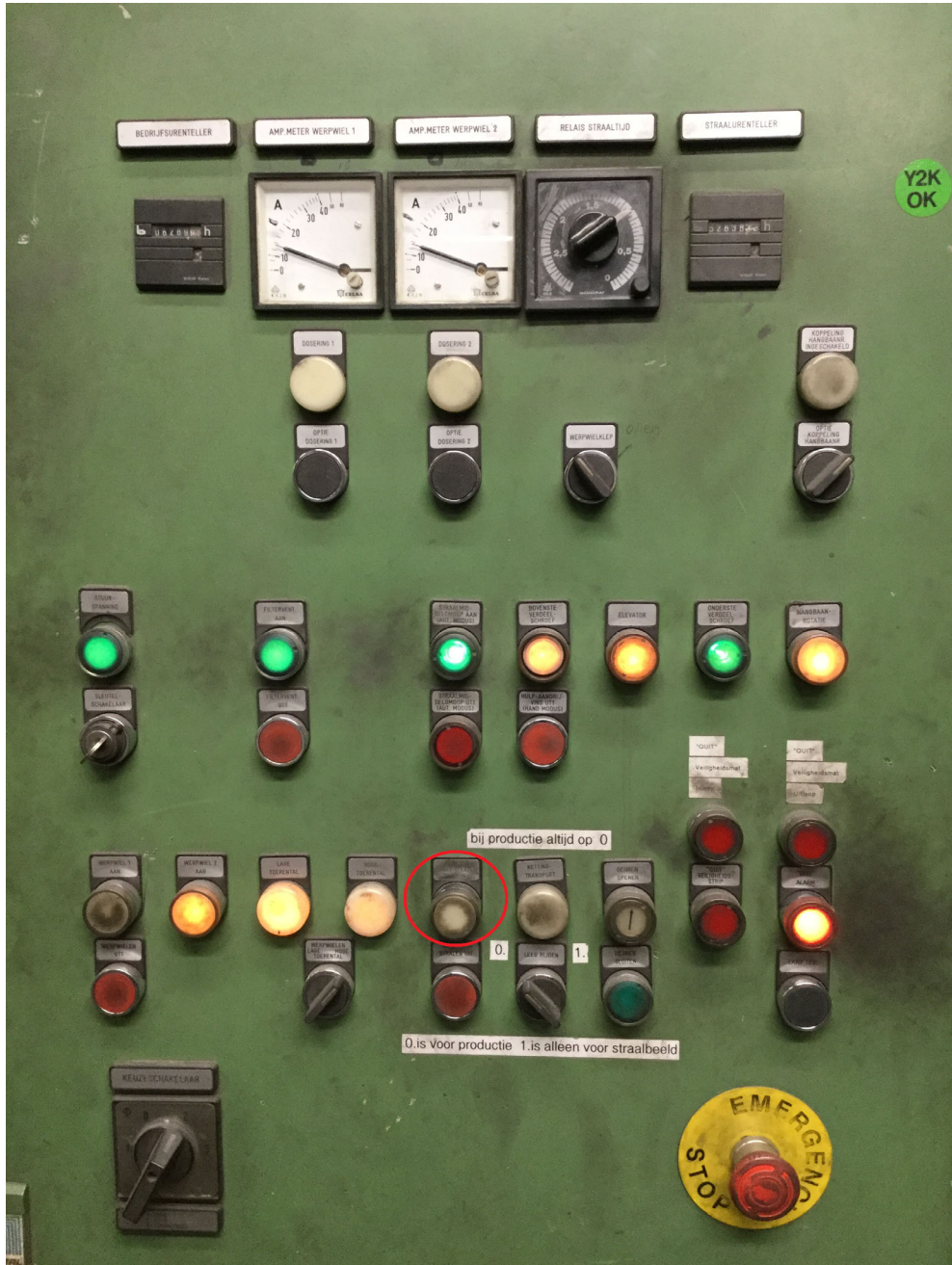
Figure 2. The control panel of the blasting machine. The “emergency stop” button is in the right bottom corner. The “start stralen” button is circled in red. [This figure appears in color in the online issue.]
